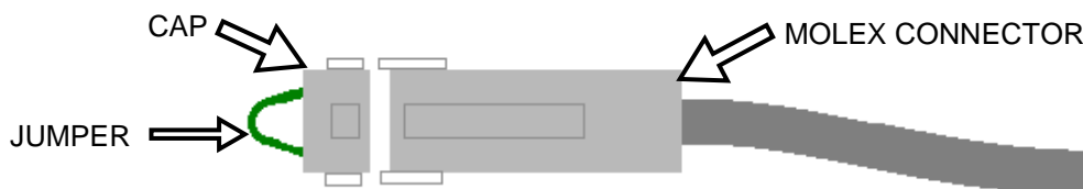
Figure 2-19: Sequencing Isolation Valve Molex Connector and Jumper Wire
