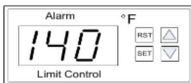
Figure 4-6: Digital Over-Temperature Alarm Switch Front Panel
