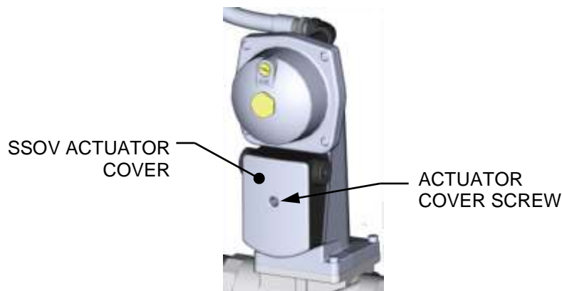
Figure 5-8: SSOV Actuator Cover Location
