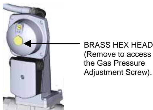
Figure 5-2: SSOV with Gas Pressure Adjustment Screw Location
