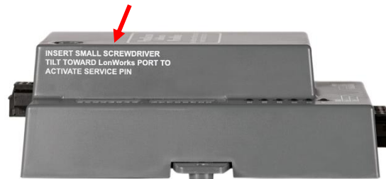
Figure 8-1: LonWorks Service Pin Location
