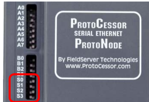
S Bank DIP Switch Location
