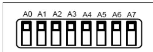
Figure 2-7: MAC Address DIP Switches
