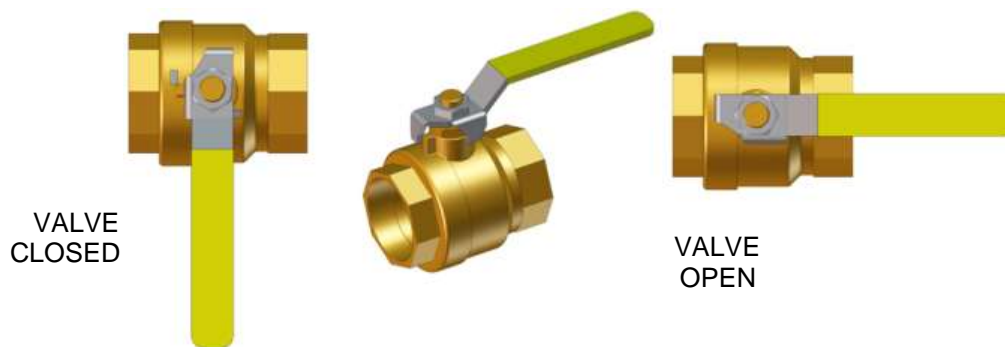
Figure 1-1: External Manual Gas Shutoff Valve
