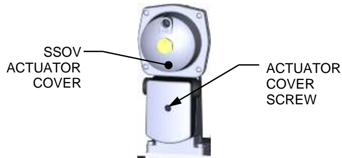
Figure 5-9: SSOV Actuator Cover Location
