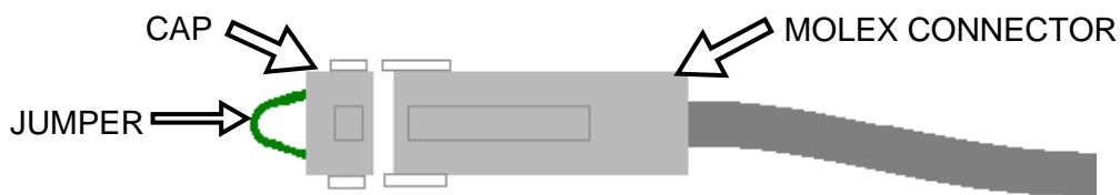
Figure 2-15a: Sequencing Isolation Valve Molex Connector and Jumper Wire
