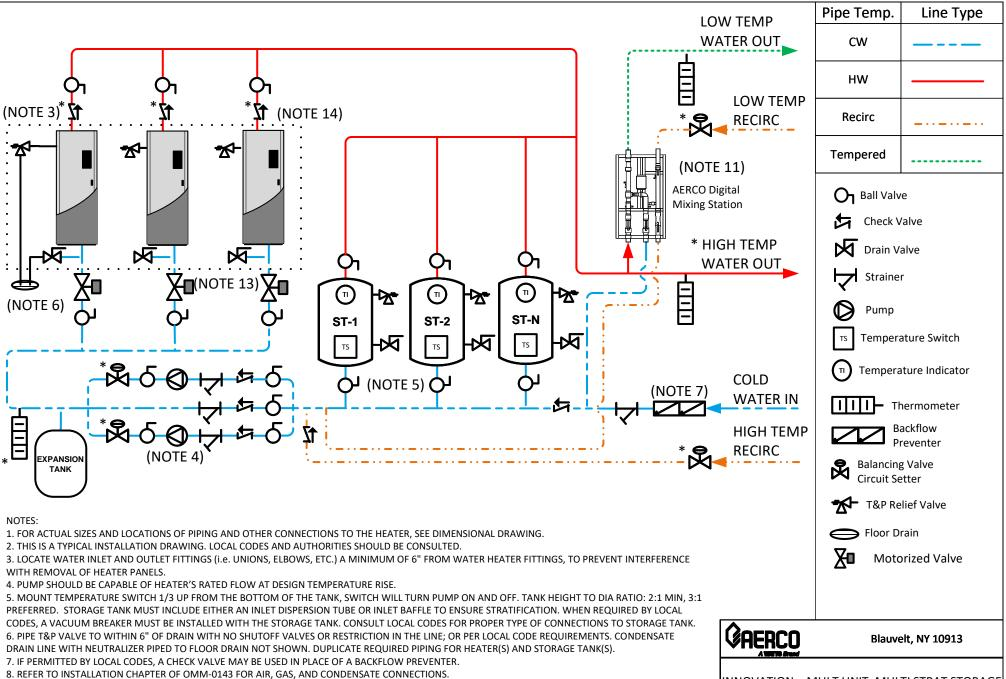
10. THE FOLLOWING COMPONENTS SHALL BE FIELD SOURCED: CHECK VALVES, STRAINERS, BALL VALVES, BALANCING VALVES, PUMPS, TEMPERATURE SENSORS, EXPANSION TANK, BACKFLOW PREVENTER. 11. BUILDING RECIRC PUMP DETERMINED BY PLUMBING ENGINEER AND MINIMUM FLOW VARIES BY DIGITEMP MODEL.
