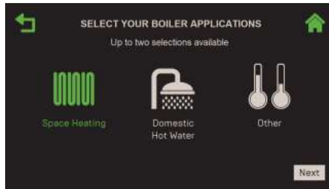
Figure 2-42: BST Manager – Space Heating: Select Your Boiler Application
