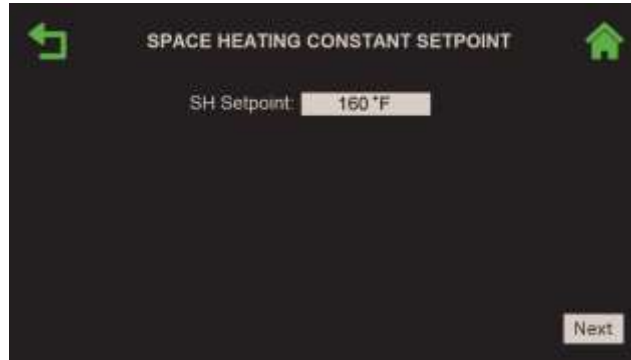
Figure 2-44: BST Manager – Space Heating: Constant Setpoint Screen
