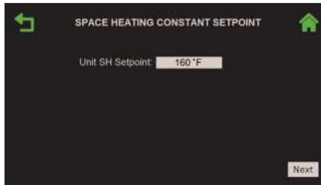
Figure 2-9: Standalone – Space Heating: Space Heating Constant Setpoint
