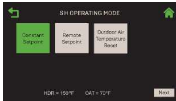
Figure 2-61: BST Manager – SH & DHW : SH Operating Mode Screen
