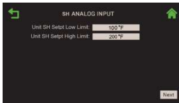
Figure 2-11: Standalone – Space Heating: SH Analog Input Screen
