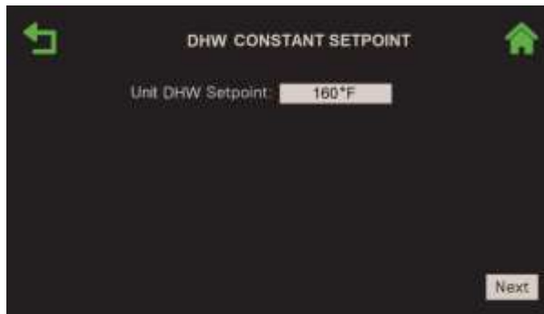
Figure 2-18: Standalone – DHW : DHW Constant Setpoint Screen
