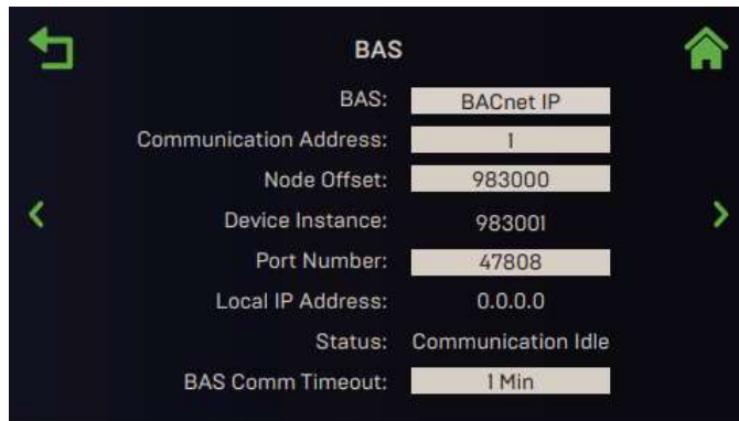
Figure 6-57a: Communication & Failsafe : BAS Screen, BAS = BACnet IP
