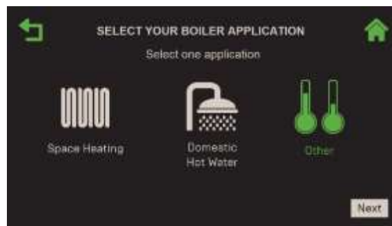
Figure 2-22: Standalone – Other: Select Your Boiler Application Screen
