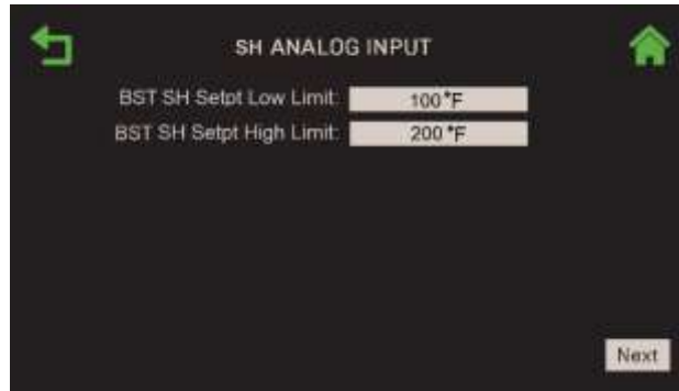
Figure 2-46: BST Manager – Space Heating: SH Analog Input Screen
