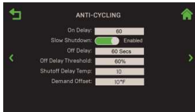
Figure 6-41: Operating Controls: Anti-Cycling Control Screen
