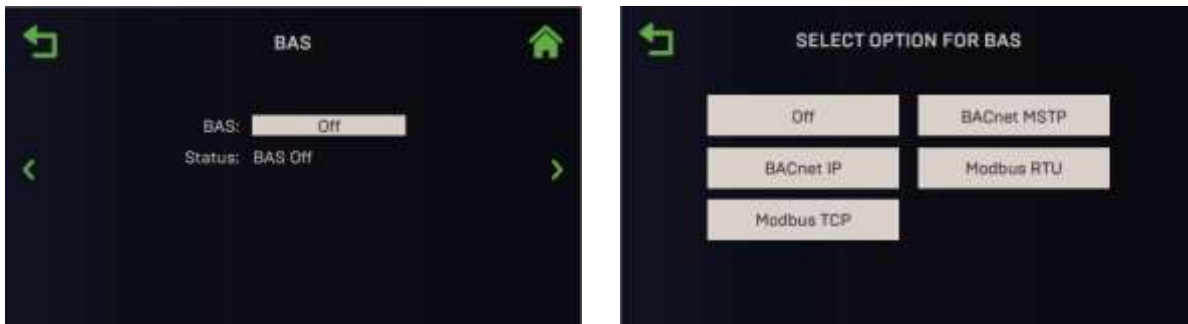
Figure 6-56: Communication & Failsafe: BAS Screens
