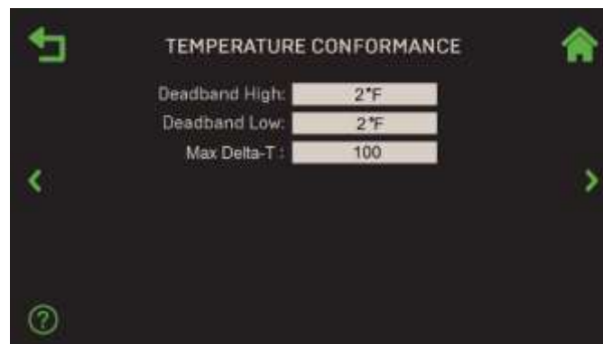
Figure 6-77: Temperature Control: Temperature Conformance
