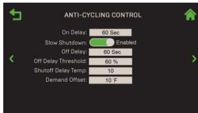
Figure 6-83: Fire Control : Standalone Anti-Cycling Controls
