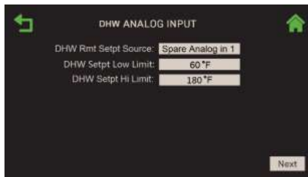
Figure 2-70: BST Manager – SH & DHW : DHW Analog Input Screen
