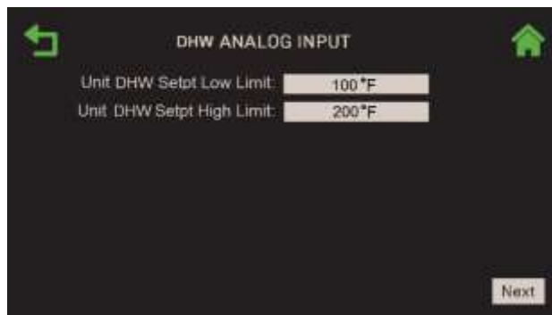
Figure 2-20: Standalone – DHW : DHW Analog Input Screen
