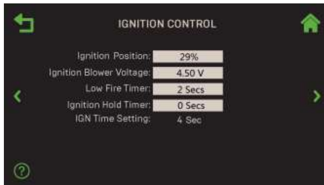
Figure 6-81: Fire Control : Ignition Control
