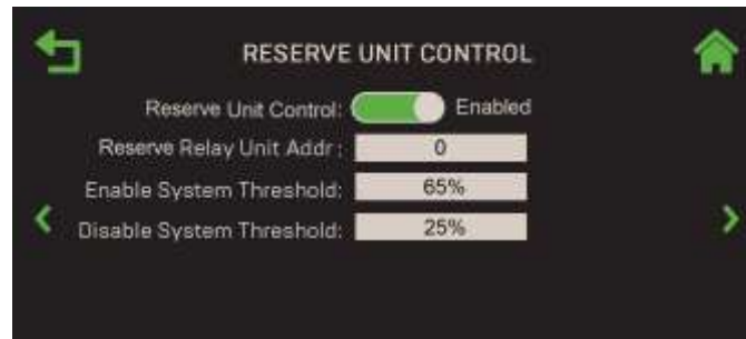
Figure 6-44: Operating Controls : Reserve Unit Control Screen
