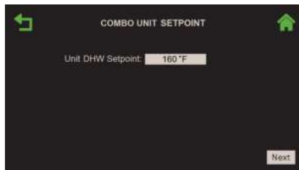
Figure 2-14: Standalone – Space Heating: Combo Unit Setpoint Screen
