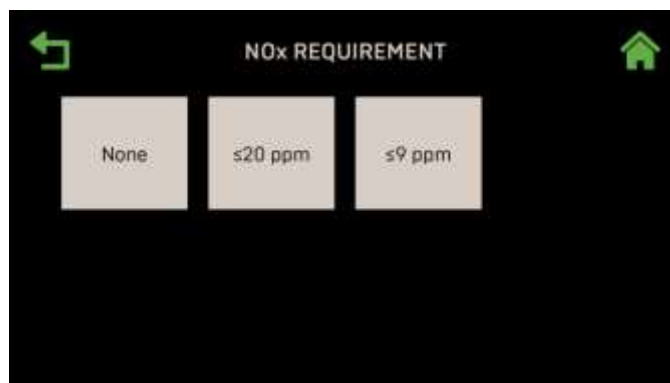
Figure 3-6: Manual Combustion : NOx Requirement Screen
