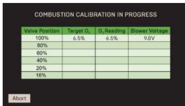
Figure 3-4: Assisted Combustion: Combustion Calibration In Progress Screen
