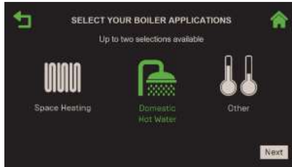
Figure 2-49: BST Manager – DHW : Select Your Boiler Application
