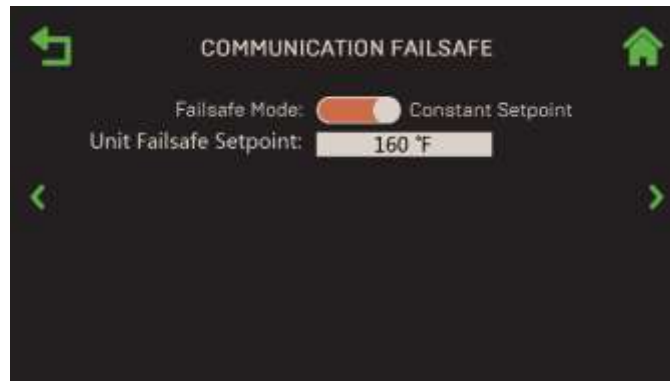
Figure 6-64: Communication & Failsafe: Communication Failsafe Screen
