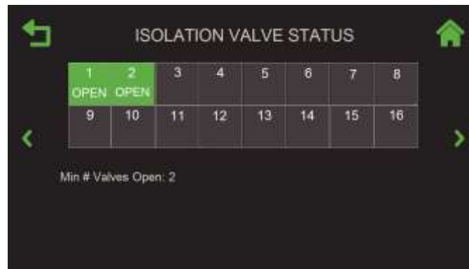
Figure 7-12: Isolation Valve Status Screen
