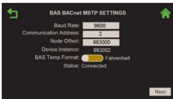
Figure 2-94: BAS BACnet MSTP Settings Screen
