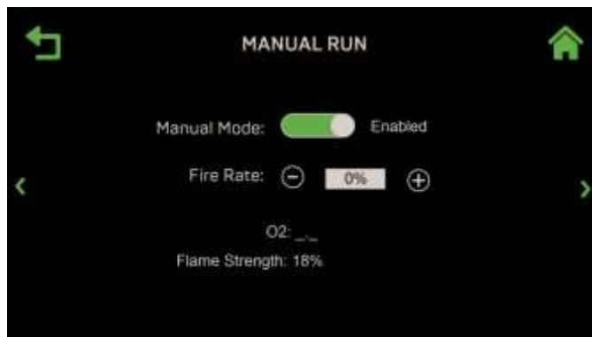
Figure 4-2: Diagnostics: Manual Run Screen – Manual Mode Enabled
