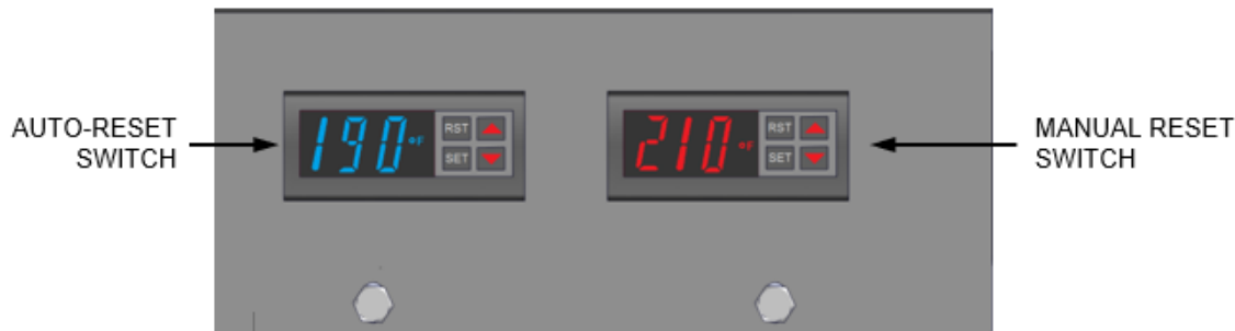
Figure 4-6: Over-Temperature Limit Switches
