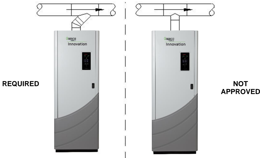
Figure 11a: Recommended Connections to Common Vent Breeching
