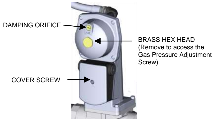
Figure 5-3: SSOV Actuator With Gas Pressure Adjustment (SKP25)
