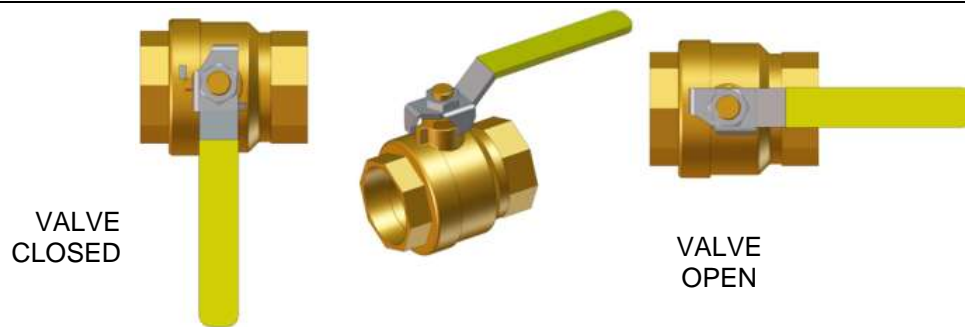
Figure 1-1: Manual Gas Shutoff Valve
