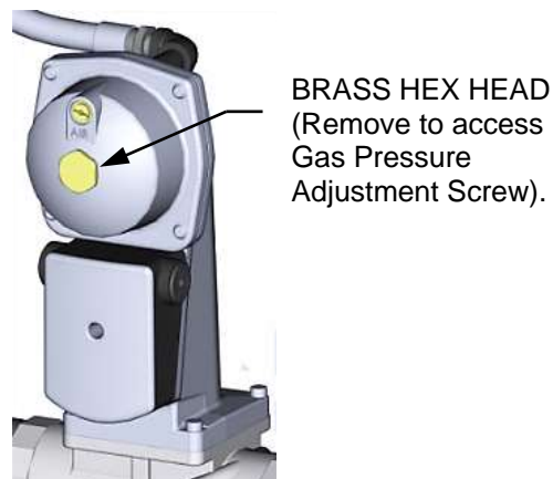
Figure 4-3: Gas Pressure Adjustment Screw Location
