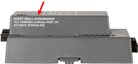
Figure 7-1: LonWorks Service Pin Location
