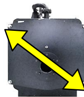
Figure 3-5: Switching Upper Left and Lower Right Bolts
