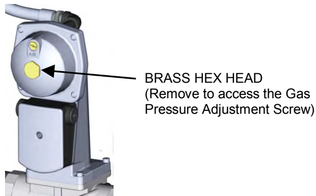
Figure 4-3: Gas Pressure Adjustment Screw Location
