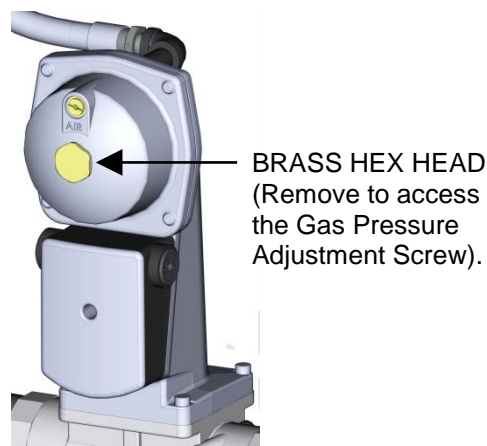
Figure 4-3: Gas Pressure Adjustment Screw Location
