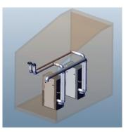
Individual sidewall vent/ common sidewall air
