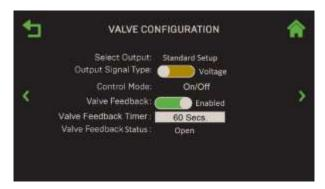
Figure 8.6-6: Operating Controls: Valve Configuration Screen
