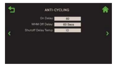
Figure 8.6-5: Operating Controls: Anti-Cycling Control Screen
