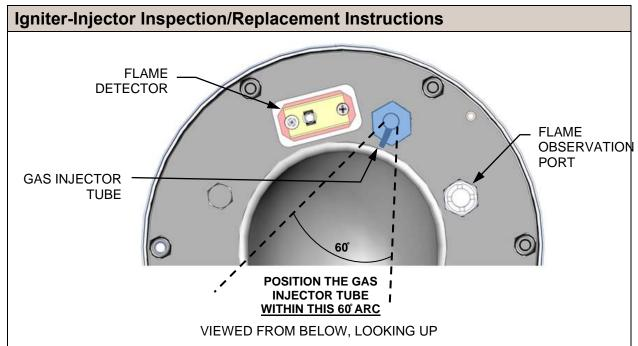
Figure 6.3-2: Igniter-Injector & Flame Detector Mounting Details
