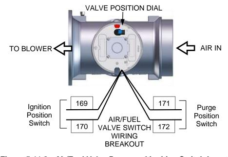
Figure 5.11-2: Air/Fuel Valve Purge and Ignition Switch Locations
