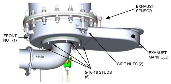
PARTIAL RIGHT-SIDE VIEW WITH SUPPORT REMOVED
