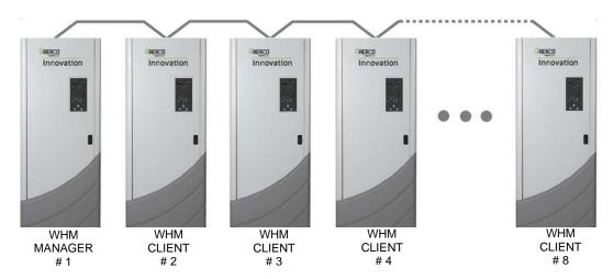
Figure 8.7.3: Typical Daisy-Chain Modbus/RS485 Network
