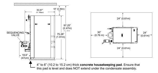
Figure 2.4.1-1: Innovation Water Heater Clearances
