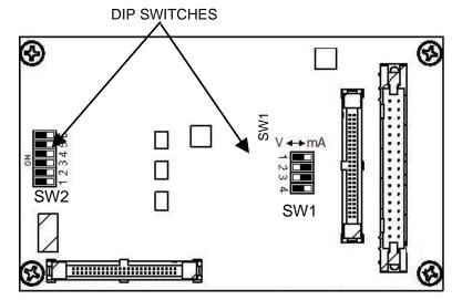
Figure G-3: Edge [i] Controller Interface Board (Behind Front Face)
