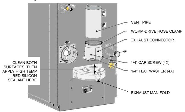
Figure 2.13. Exhaust Vent Connection
