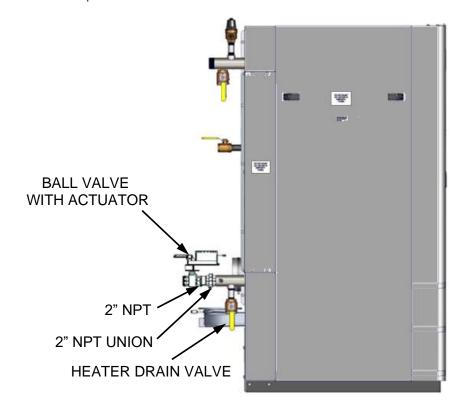
Figure 2.5.1: Innovation Water Heater Equipped with Sequencing Valve
