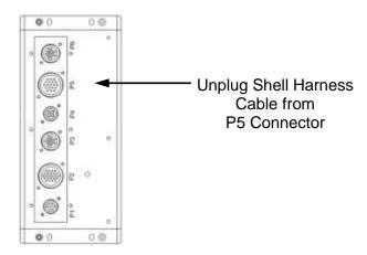
Figure 6.11.1-1: Removing Shell Harness Cable from P5 Connector on Rear Panel
