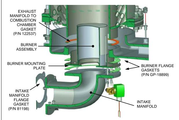
Figure 6.7-2: Intake Manifold and Burner - Cross-Section, Exploded
