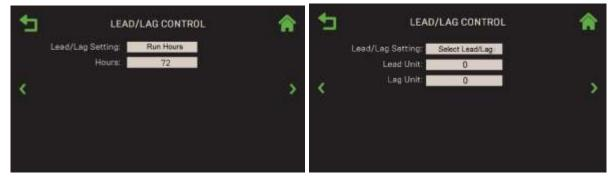
Figure 8.6-7: Operating Controls: Lead/Lag Control Screen
