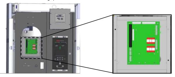
Figure 2.12-1: Input/Output (I/O) Box Location – Partial Front View
