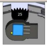
Figure 3.4-4: 25% Air/Fuel Valve Ignition Position
