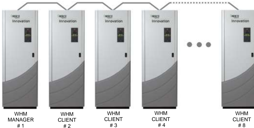
Figure 8-3. Typical Daisy-Chain Modbus/RS485 Network
