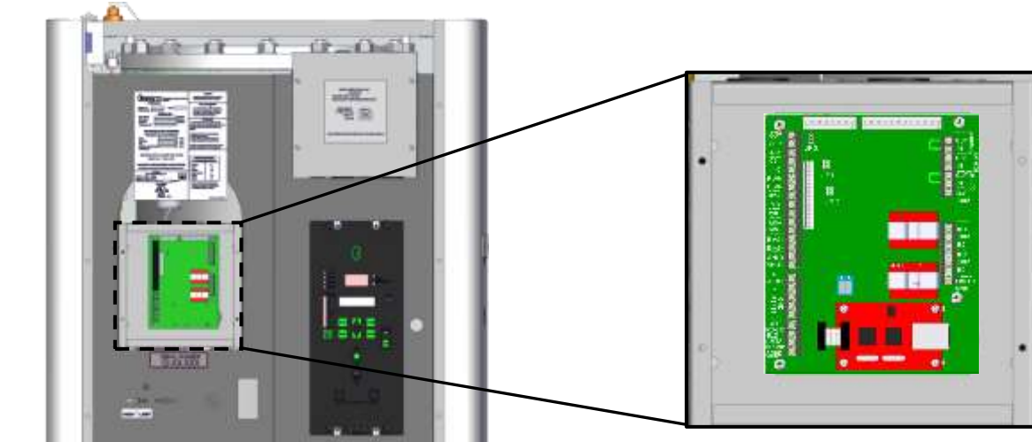
Figure 2-12. Input/Output (I/O) Box Location – Partial Front View
