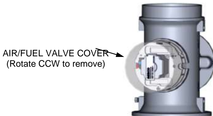
Figure 5-7. Typical Air/Fuel Valve Cover Location
