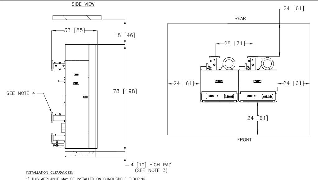
1) THIS APPLIANCE MAY BE INSTALLED ON COMBUSTIBLE FLOORING 2) MINIMUM CLEARANCES TO ADJACENT CONSTRUCTION ARE AS FOLLOWS:
