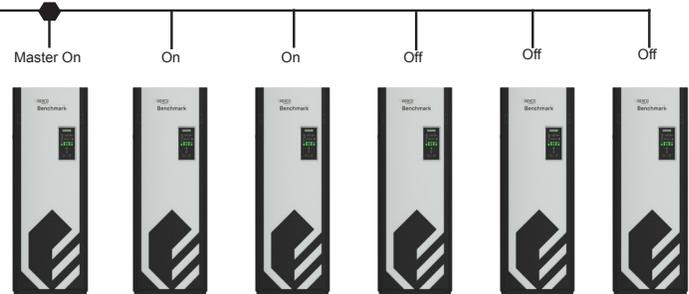
Importantly, because the BST reacts in real-time to, up to 8 boilers, changes in the number of boilers available, users can take a unit offline for maintenance at any time or bring on back-up boilers for extremely cold conditions without changes to the BST. And as individual boilers are added or deleted, the energy delivered is automatically adjusted to prevent fluctuations in the header temperature of the plant.
