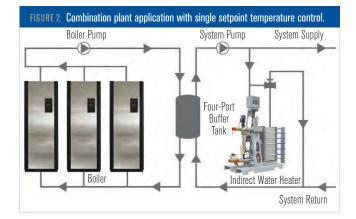
This design adds a layer of security, as well. For example, if the DHW boiler cannot meet its load, the controller will direct the swing valves to divert its designated boilers from space heating to DHW. As per ASHRAE, it is assumed that both space heating and DHW peak loads may not happen concurrently.<sup>3</sup> This offers a major benefit in reducing the number of boilers required to meet plant peak load, shrinking the footprint.
