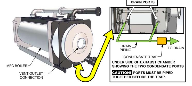
Figure 1: Location and Piping of the Two Condensate Drain Ports
