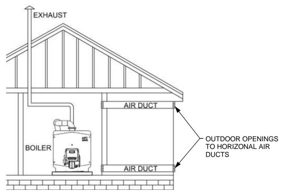
Figure 5: All Combustion Air from Outdoors through Horizontal Ducts
