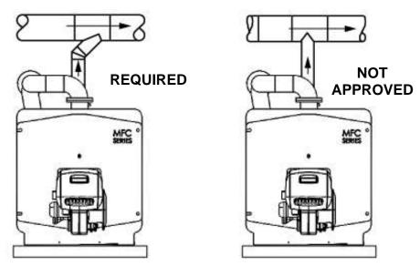
Figure 9a: Recommended Connections to Common Vent Breeching
