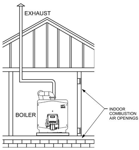
Figure 2: All Combustion Air from Adjacent Indoor Spaces through Indoor Combustion Air Openings
