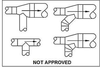
Figure 10: Required Transition Vent Sections
