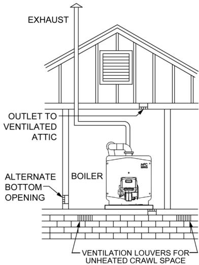
Figure 3: All Combustion Air From Outdoors - Inlet Air From Ventilated Crawl
