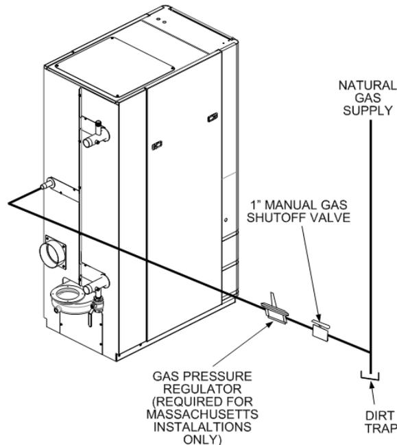
**Figure 2-8. Manual Gas Shut-Off Valve Location**
