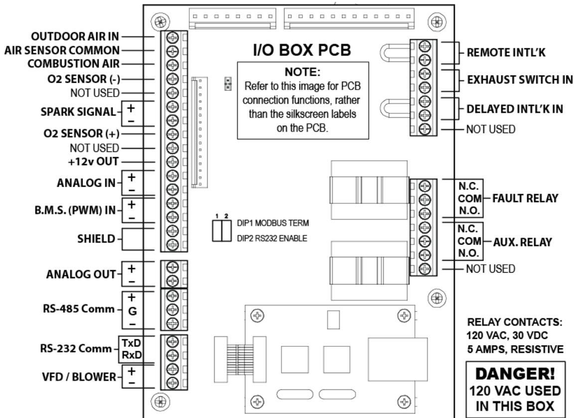
**Figure 2-12. I/O Box Terminal Strips**
