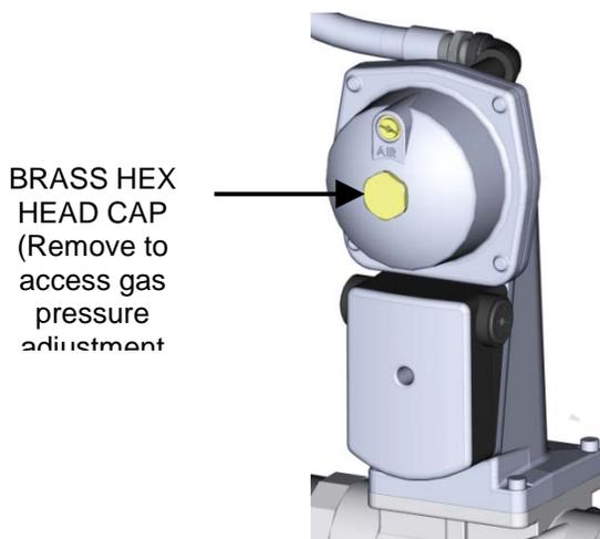
**Figure 4-4. Gas Pressure Adjustment Screw Location**
