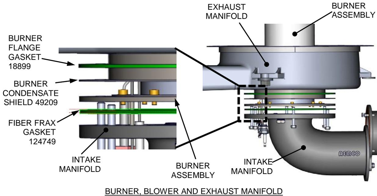
**Figure 6-6. Combustion Chamber Liner & Gasket Locations**
