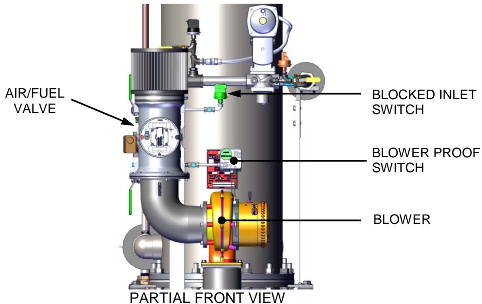
**Figure 5-4. Blower Proof & Blocked Inlet Switch Locations**
