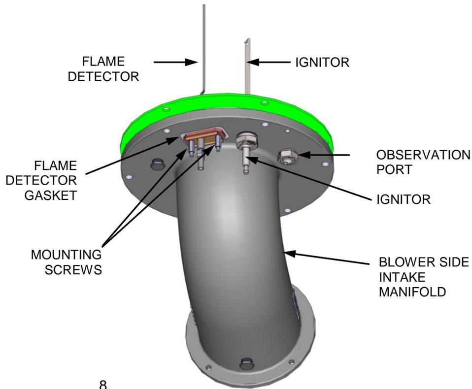
**Figure 6-2. Igniter & Flame Detector Mounting Details**
