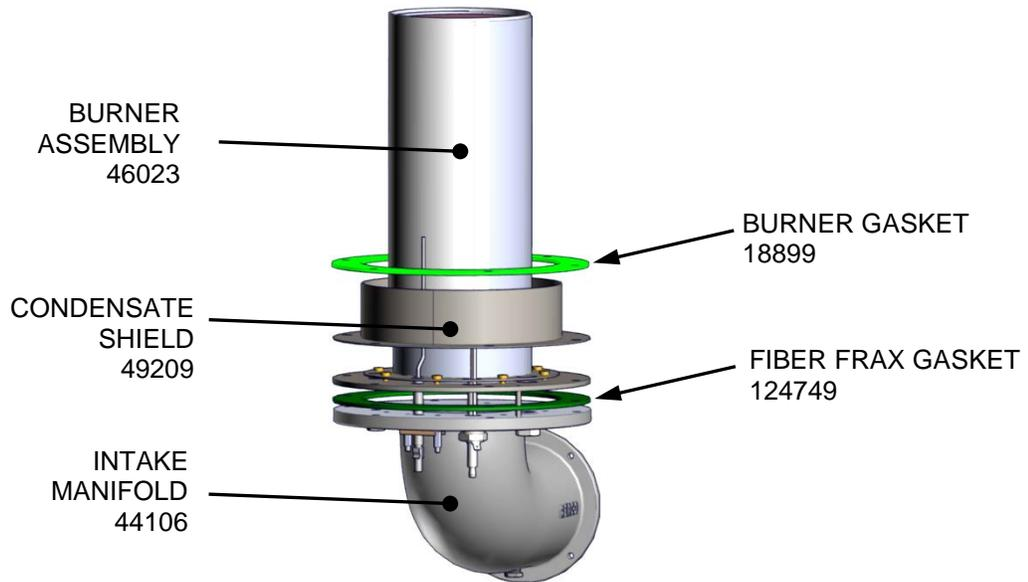
Figure 6-4. Innovation Heater – Partial Left-Side View
