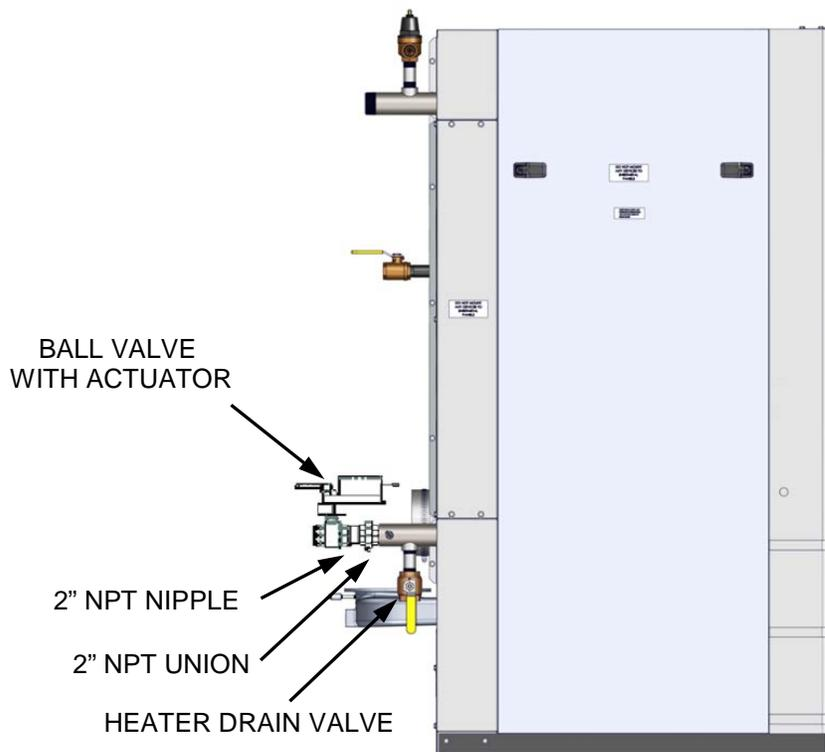
**Figure 2-3b. Innovation Water Heater Equipped With Sequencing Valve**
