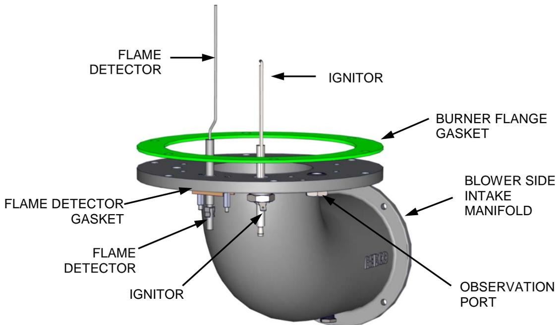
Figure 7-2. Blower-Side Intake Manifold (Shown removed from Heater)
