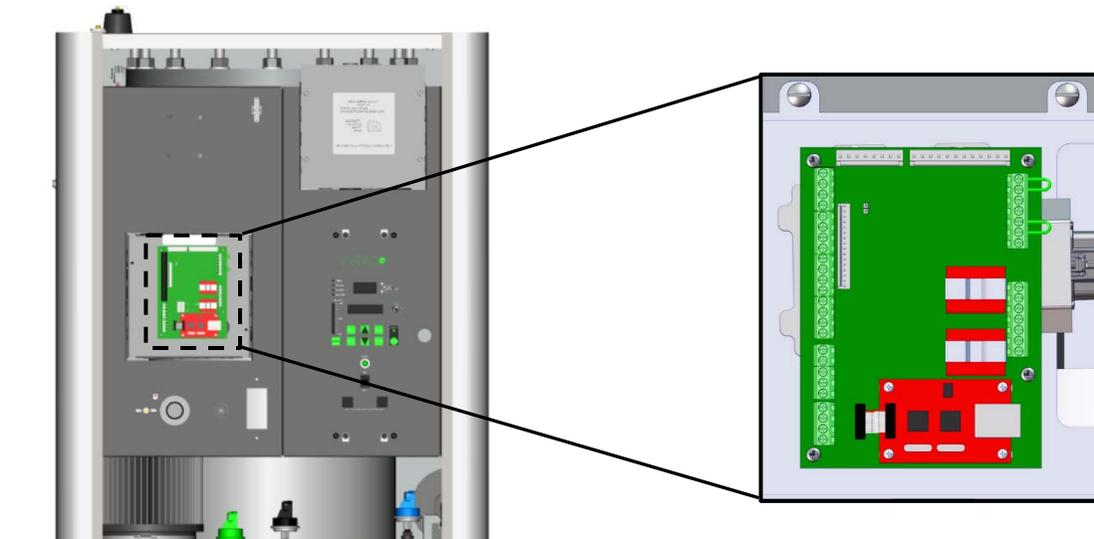
**Figure 2-11. Input/Output (I/O) Box Location – Partial Front View**
