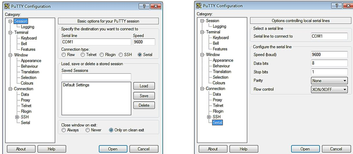
**Figure 8-1: PuTTY GUI: Basic Serial Session (L) and Serial Options (R)**
