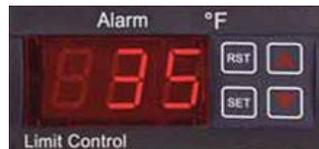
**Figure 8-28. Over-Temperature Switch & Temperature Indicator**
