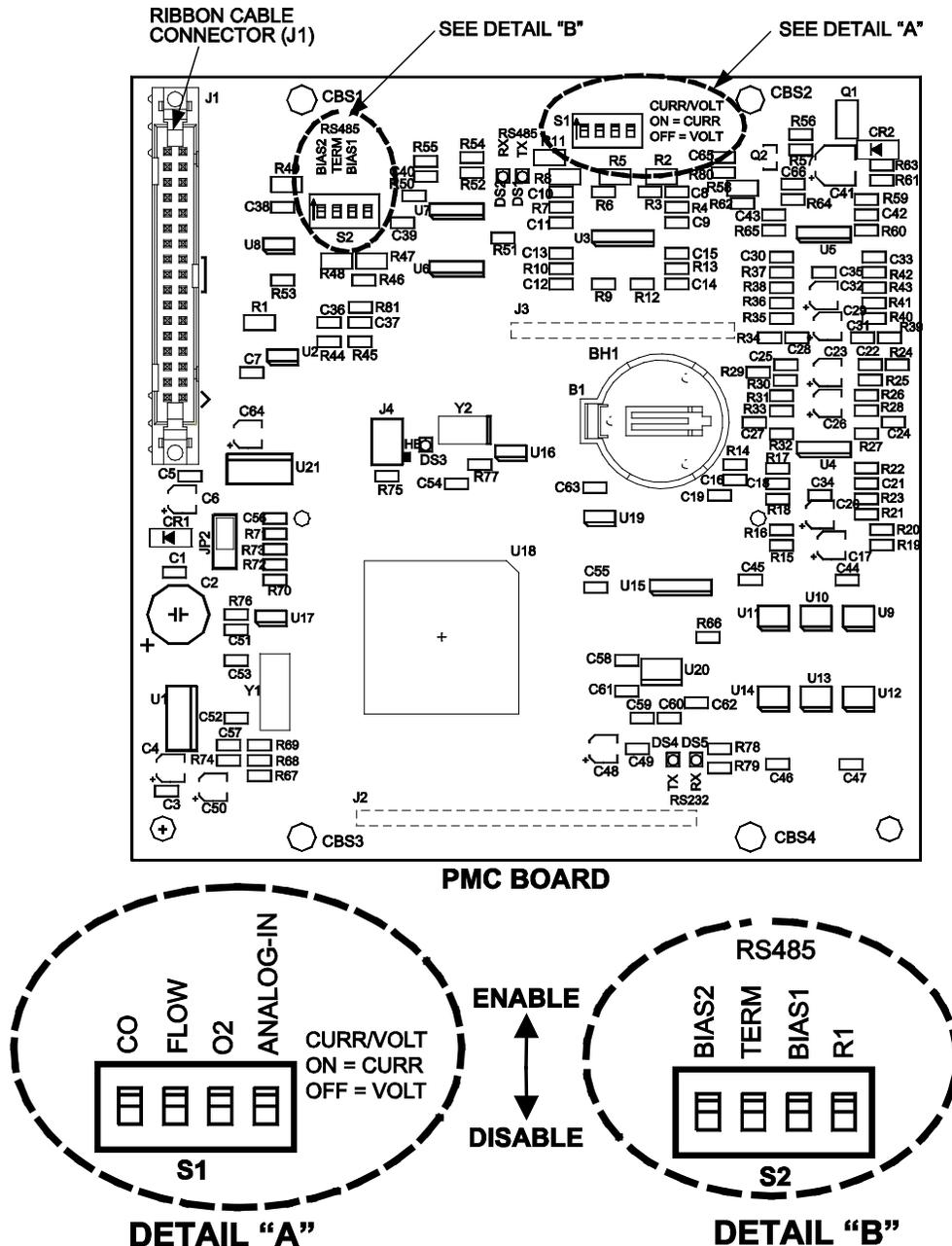
**S1:** These DIP Switches are used to set either current (CURR) or voltage (VOLT) as the remote signal input source.
