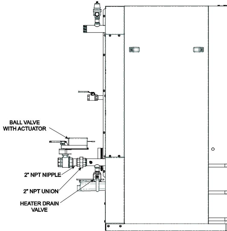
**Figure 8-2. Innovation Water Heater Equipped With Sequencing Valve**
