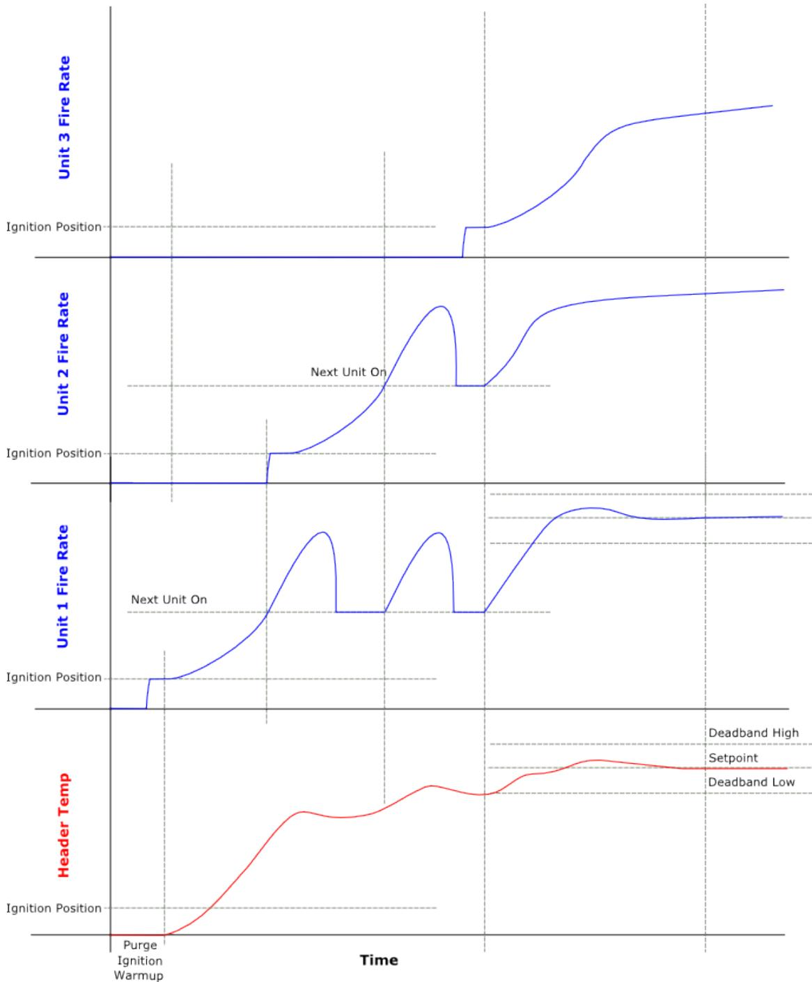
**Figure9.2: BST Multiple Boiler Sequence Of Operation – 2 of 2**
