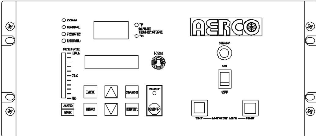
**Figure 1-1B. C-More Control Panel For KC1000 Series Units**
