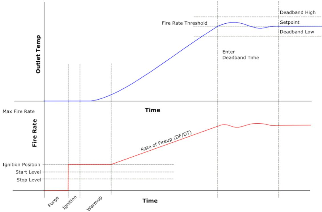
**Figure 9-2: BST Single Boiler Sequence of Operation – 1 of 2**
