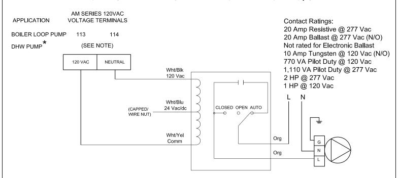
MANUFACTURER: FUNCTIONAL DEVICES RELAY MODEL: RIB2401SB
