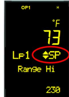
3. Press until the **Alternate Setpoint Enable (Alt SP En)** is displayed.
