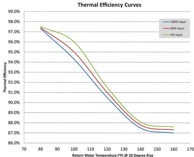
Since the majority of a boiler's operating hours will be under “part load conditions,” modulating units promise greater seasonal efficiency.
