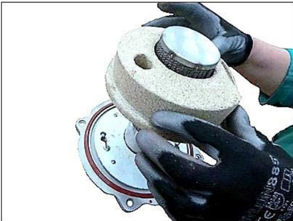
**Figure G: Remove Thermal Insulation**
