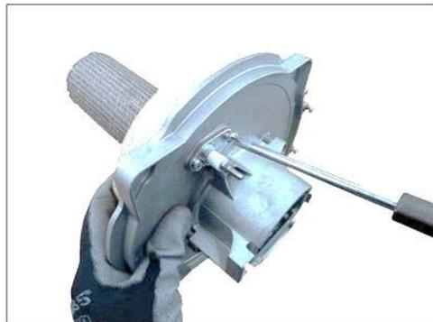
**Figure L: Tighten the Electrodes**
